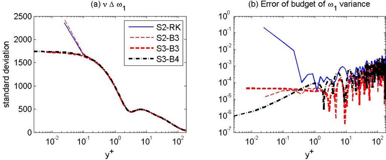
Figure 2: Statistical results for different cases in the domain with length  $L = 4\pi$ . Thin blue solid: S2-RK; Thin red dashed: S2-B3; Thick red dashed: S3-B3; Thick black dash-dotted: S4-B3. (a): Standard deviation of  $\nu\Delta\omega_1$ . (b): Relative error of the budget of the variance of  $\omega_1$ .
